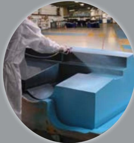
Protectapeel was used to protect bare steel parts on sections of the Queen Elizabeth Carrier as they were made.
