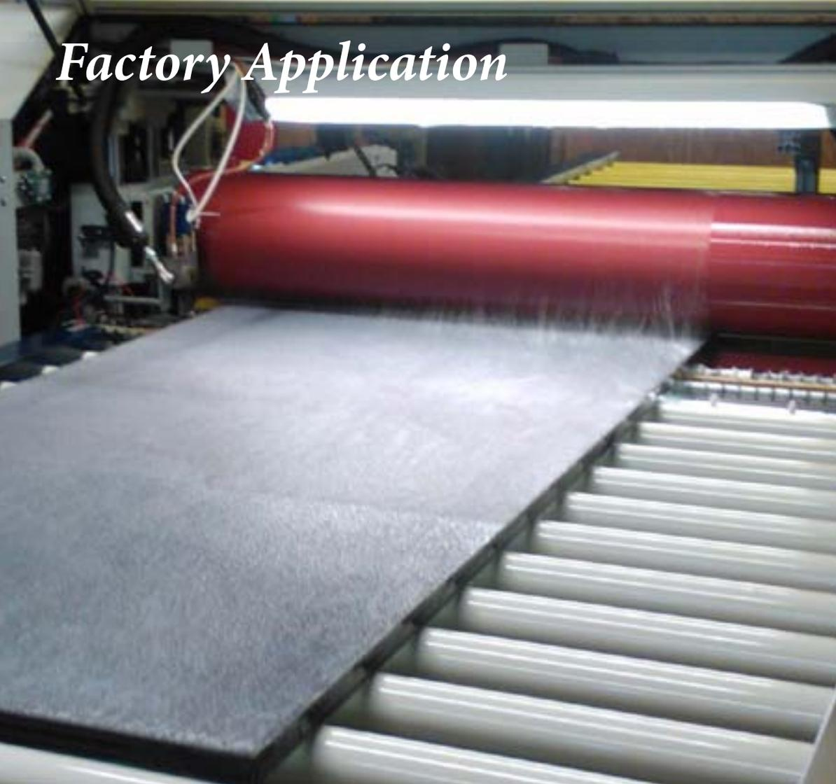
Protectapeel offers a range of instant cure, weather resistant, peelable protective coatings for glass and non-porous substrates. The coatings are suitable for factory application and in-line manufacturing processes, providing tough protection during storage, transportation and installation against:
