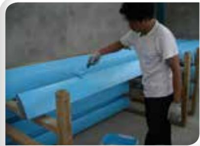
These anodised aluminium bull nose cills were used on the Shanghai Financial Centre. Protectapeel was rolled onto the surface using a lambs wool roller.
