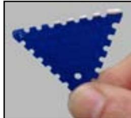
**6.** Use a wet film gauge to check the coatings wet film thickness; make sure this is the same minimum WFT as stated in the product's Technical data sheet (TDS). Remove any masking tape whilst the product is still wet.
